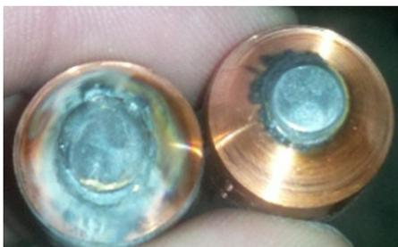
The WTC control can measure precise resistances of welding tips after they have been dressed. Although dressers can remove slag from the edges, the control will identify if the surface of the electrodes are brought back to an approved condition.
