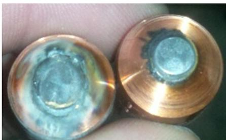
The WTC control can measure precise resistances of welding tips after they have been dressed. Although dressers can remove slag from the edges, the control will identify if the surface of the electrodes are brought back to an approved condition.
