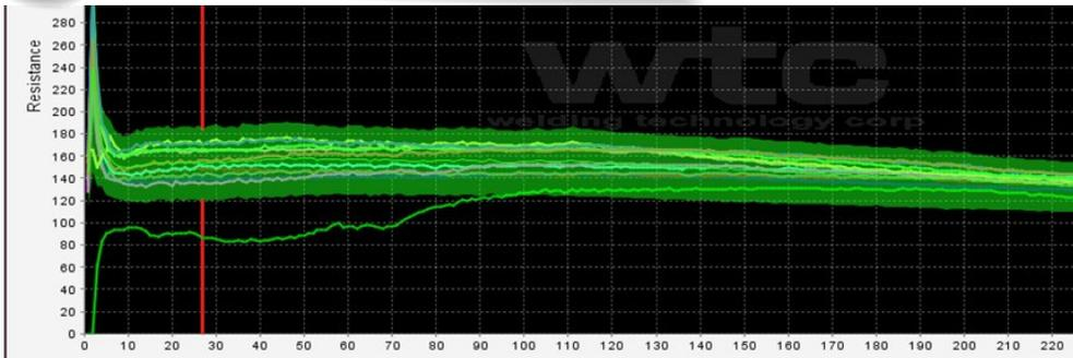
Keep your process consistent using signature analysis for each and every weld. With the View-R Network concentrator, you can report these excursions by control, by machine, and by part.
